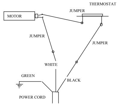
**NOTE:** "If any of the original wire supplied with the appliance must be replaced, it must be replaced with a wire of at least a 105° C. temperature rating.
